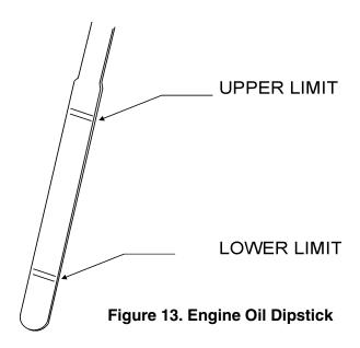
When checking the engine oil, be sure to check if the oil is clean and viscous. If the oil is not clean, drain the oil by removing the oil drain plug, and refill with the specified amount of oil as outlined in the Kubota Engine Owner's Manual.
